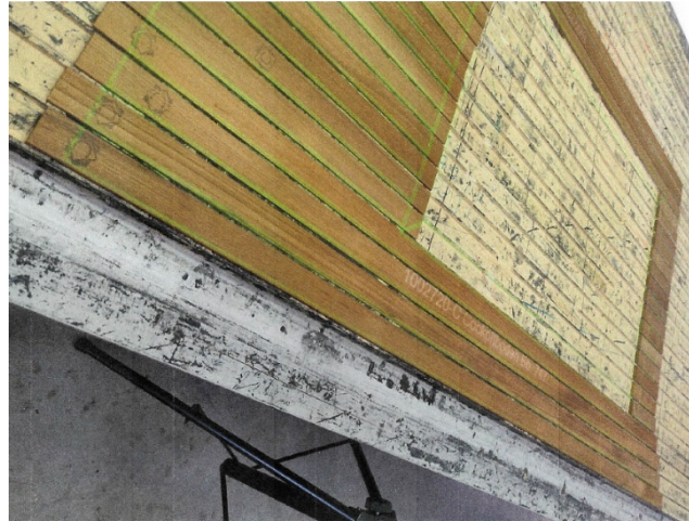
Figure 4. Digital placement templates in boat building: Projection replaces physical templates and enables precise, time-efficient placement of rod decks directly on the work surface.
