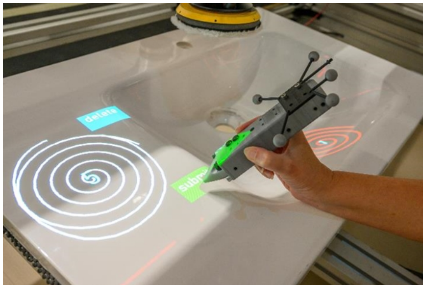
Figure 1. Order generation for spot processing of washbasins
